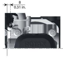
position temperature sensor new configuration
